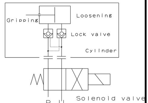
The gripping position must be retained.
