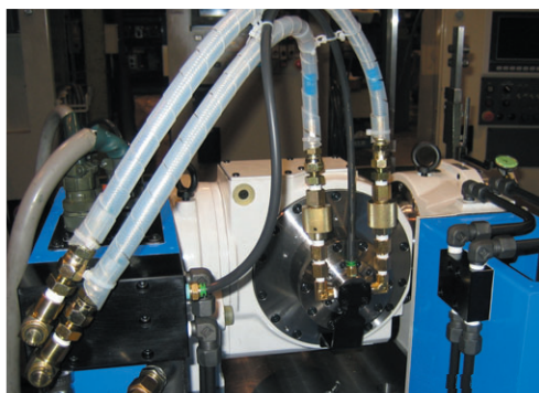
● Simplified pipework with complete built-in rotary joint (option)
