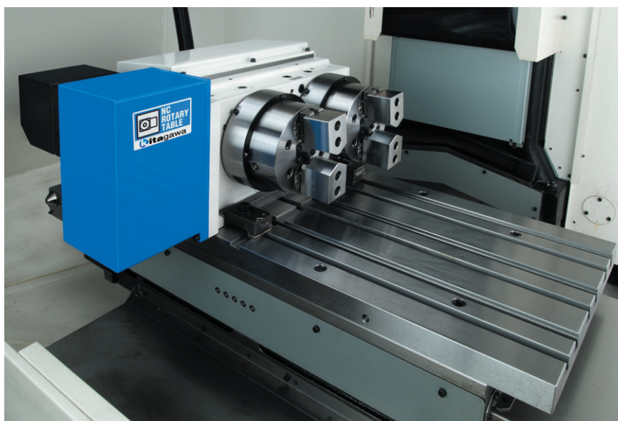
▲Work holding device combining NC Rotary Table and Chuck.
