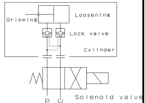
The gripping position must be retained.
