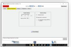
**Settings Tab** displays grip force in newtons, kilograms force and pound force. It also has settings to disable or enable data collection and create and save a sensor log file.
